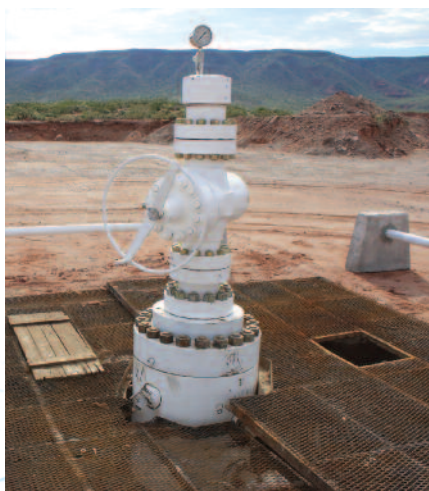
Wellhead on a site owned by Total in Auca Mahuida. © Observatorio Petrolero Sur
