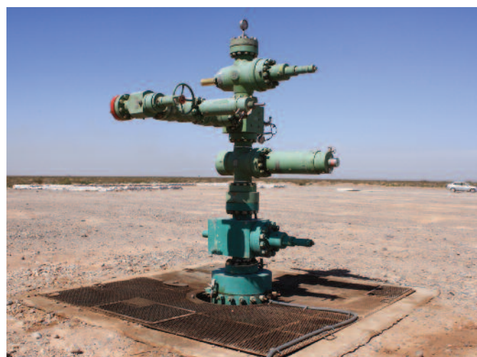
Well head on a Shell drilling site in Sierras Blancas. © Observatorio Petroleo Sur
